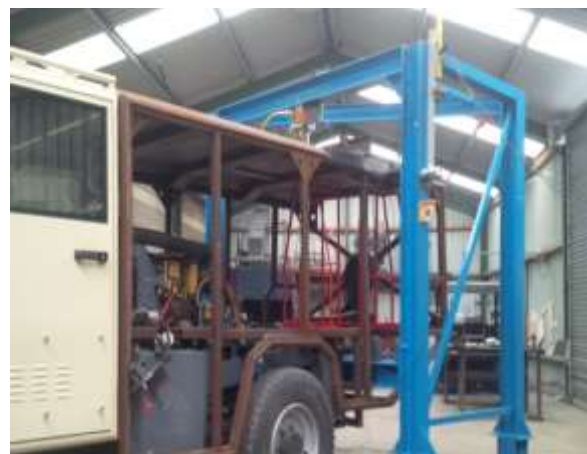
Fig: Testing Fixture for Body Frame
