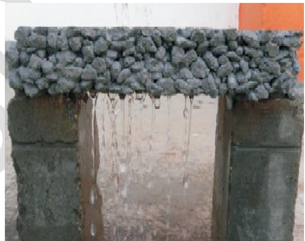
Fig 2. Pervious concrete specimen to determine the infiltration rate of water
