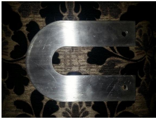
Fig. 3 Fabricated Curved Beam Specimen
