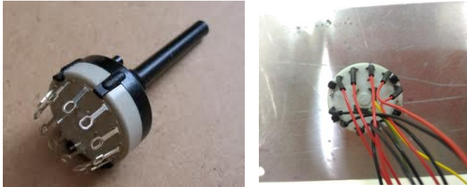
Fig. 5 6 way 2 pole switch accommodating all lead wires
