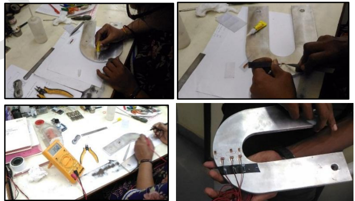
Fig. 4 Strain Gauge Mounting Procedure
