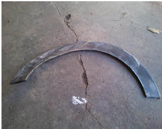
Fig. 7 Fabrication of Helical strips
