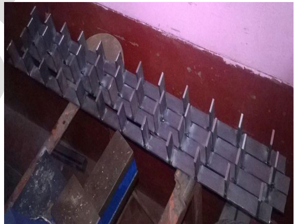
Fig. 4 Fabrication of cutter strip with blades
