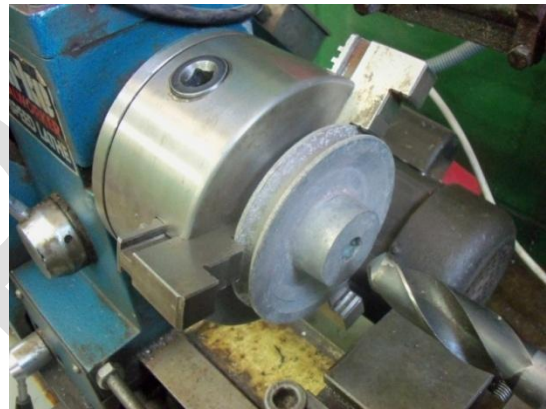
Fig. 8 Boring operation on both Pulleys
