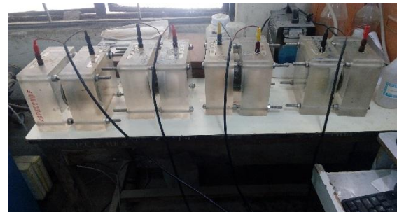
Figure 4: RCPT setup as per ASTM C120
