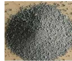
Fig. Micro concrete
