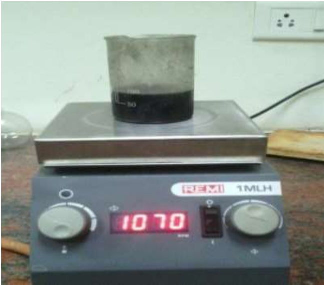
Figure.3. Dispersion of MWCNT using Magnetic Stirrer
