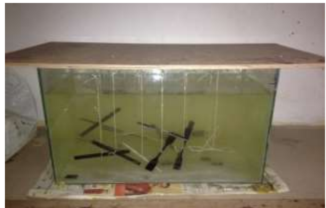
Figure.15. Immersion of specimens (with and without MWCNT) in water
