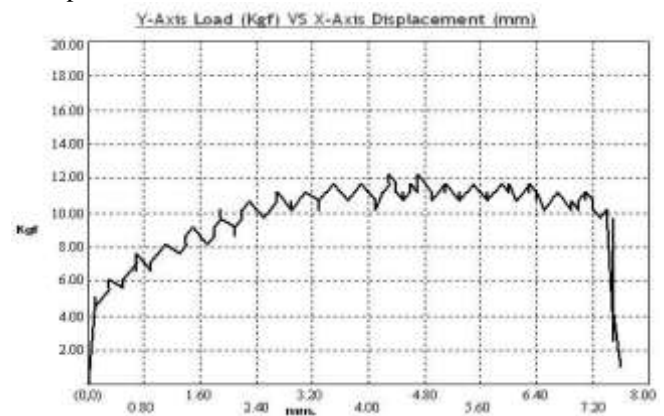
Figure.13. Load v/s Displacement for specimen
