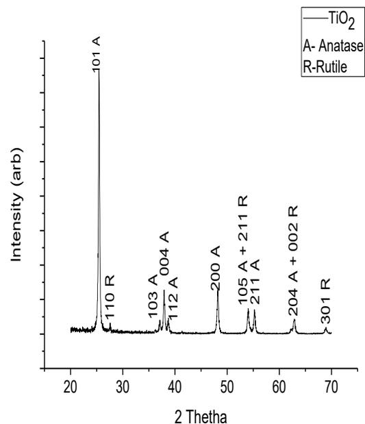
Fig. 1: X-ray diffraction pattern (XRD) of TiO<sub>2</sub> nanopowder.
