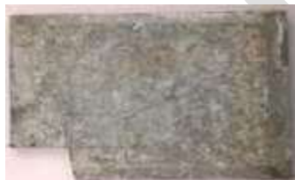
Fig 6.6(c) Zinc Corroded
