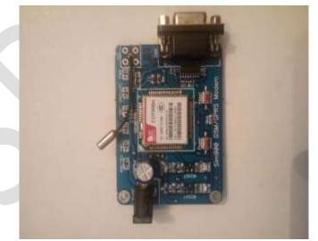
It works on frequency ranges 850/900/1800/1900 MHz It works well for SMS, voice calls and data transfer applications. [2]
