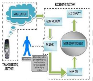
*D*. Once the message is received from the GSM modem, it is then sent to the microcontroller which processes this data.
