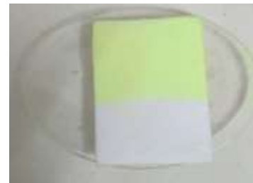
Fig 1 deposition of CdS on Teflon substrate
