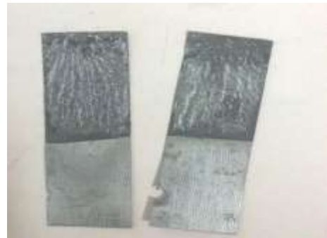
Fig.3 after deposition of CdS onto zinc substrate
