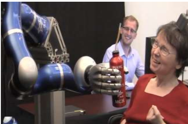
Fig4: mind controlled robotic arm serving paralyzed with a can of juice.
