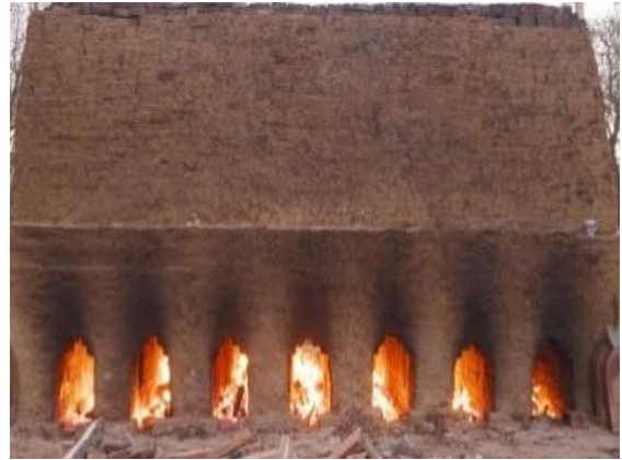
Fig 2 Burning of bricks
