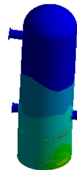
Stress due to wind load
