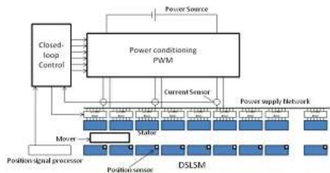
Figure 1: The basic structure of EMALS
