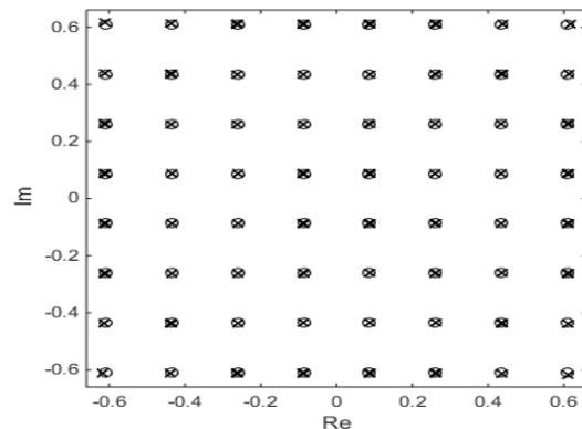
Fig. 5. Output after combined Predistorter and Wiener Model with IBO=5 dB. 'x' represents output  $y(n)$  and 'o' represents input 64-QAM signal  $x(n)$ .
