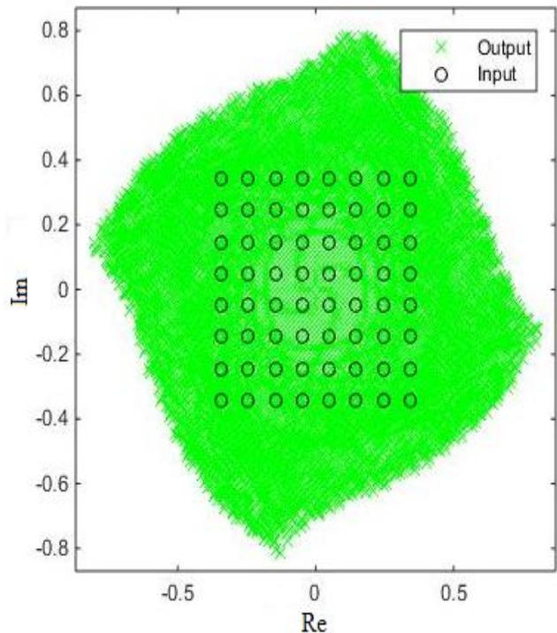
Fig. 3. Output from Wiener Model with IBO 10 dB. 'x' represents output  $y(n)$  and 'o' represents input 64-QAM signal  $x(n)$ .
