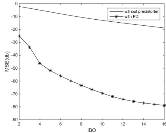
Fig. 4. MSE Vs IBO performance of designed predistorter, where wiener power amplifier is using  $h^T=[0.7692 \ 0.1538 \ 0.0769]$  and  $t^T=[2.1587 \ 1.15 \ 4.0 \ 2.1]$ .
