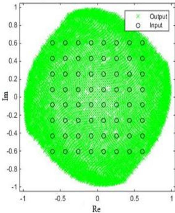
Fig. 2. Output from Wiener Model with IBO 5 dB. 'x' represents output  $y(n)$  and 'o' represents input 64-QAM signal  $x(n)$ .
