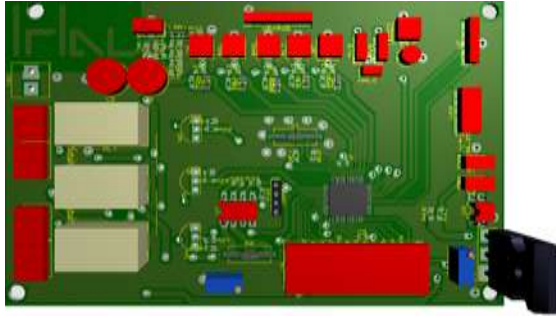
Fig 5 Solar Panel Characteristic Determining Circuit Proteus ARES Designed Circuit Top View
