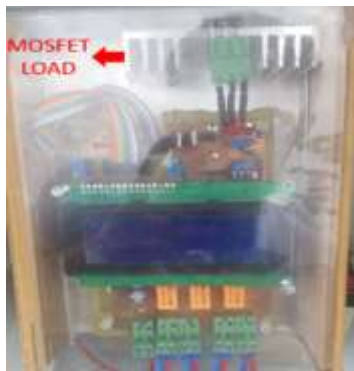
Fig 6 Implemented and Tested Solar Panel Characteristic Determining Circuit
