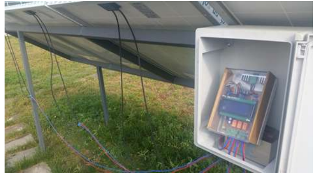
Fig. 3 Solar Panel Characteristic Determining Circuit and Solar System
