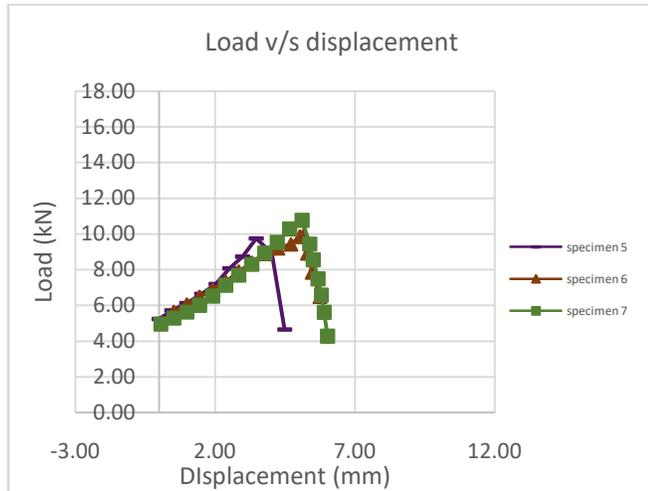
Fig. 8 Load v/s displacement for samples with filler material immersed in sea water.
