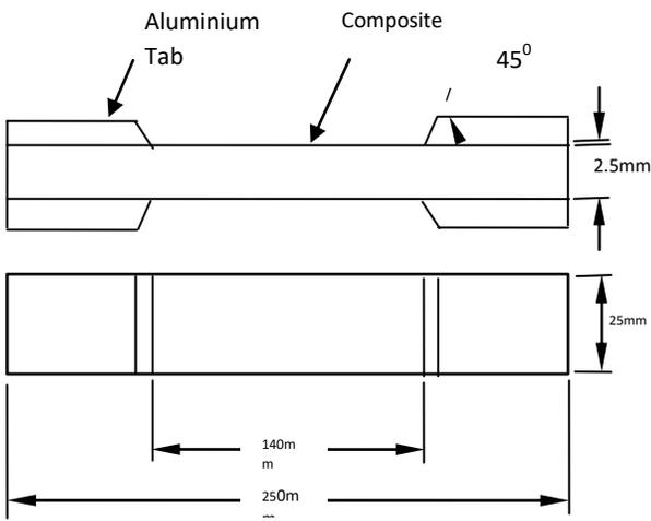
Fig. 3 Test sample as per ASTM D3039 standards.
