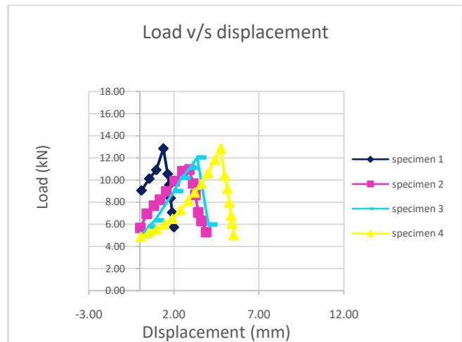
Fig. 7 Load v/s displacement for samples without filler material immersed in sea water.
