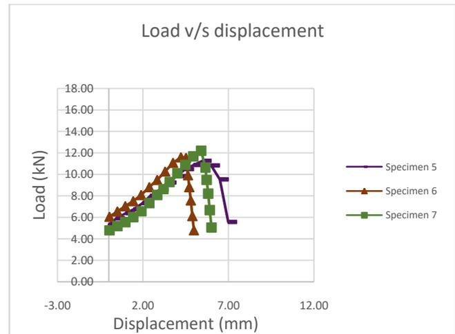
Fig. 10 Load v/s displacement for samples with filler material immersed in distilled water.
