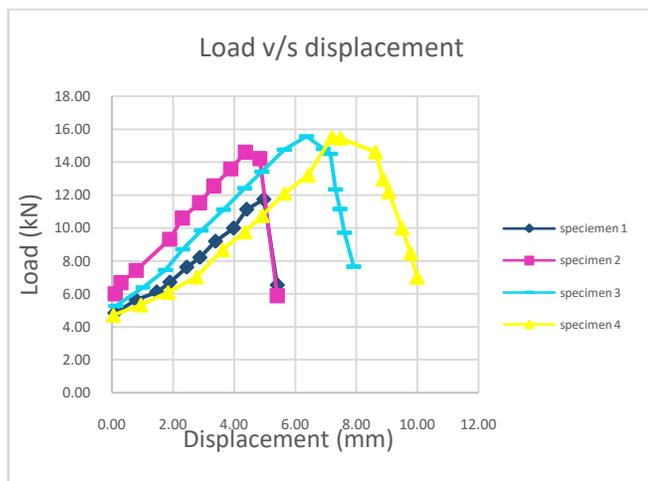
Fig. 5 Load v/s displacement for samples without filler material immersed in normal water.
