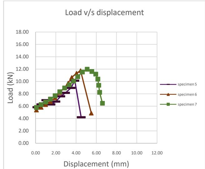
Fig. 6 Load v/s displacement for samples with filler material immersed in normal water.
