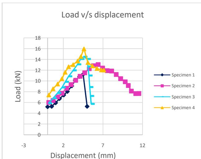
Fig. 9 Load v/s displacement for samples without filler material immersed in distilled water.
