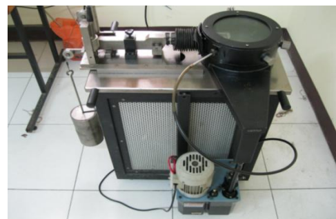
Fig. 1 Pin-on disc type wear tester
