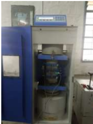
Figure 1 Testing of Specimen for Young's Modulus test
