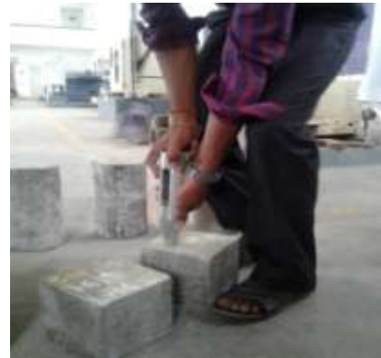
Figure 2 Rebound Hammer Test on cylindrical specimen
