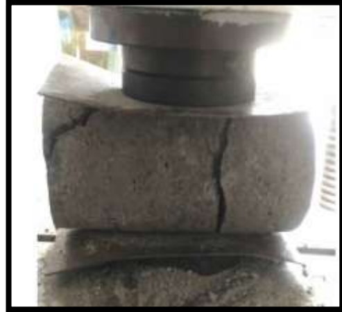
Fig 9: Split tensile test
