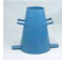
Fig 1: Slump cone apparatus
