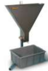
Fig 6: V-funnel test apparatus
