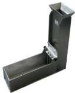
Fig 5: L box apparatus
