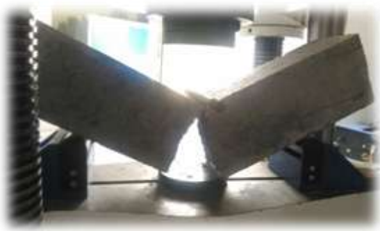
Fig 11: Flexural strength test
