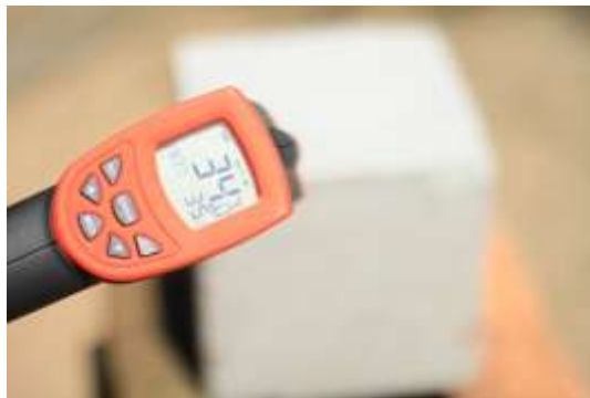
Fig.4 Measuring surface temperature
