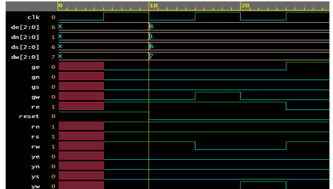
Figure 3 Simulation Result of Traffic Light Controller
