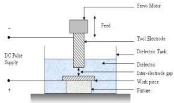
Figure 1.1: Schematic of an Electric Discharge Machining (EDM) machine tool
