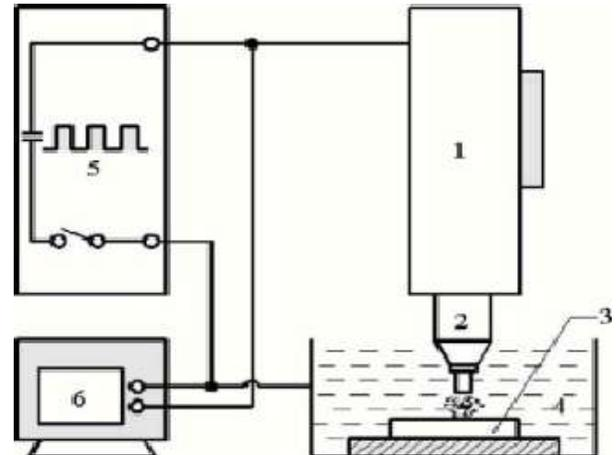
Fig. 2.1—Schematic diagram of EDM process (1- servo control, 2- electrode, 3- Specimen, 4- dielectric fluid, 5- pulse generator, 6- oscilloscope)
