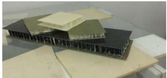
Fig 2.4.3 Composite honeycomb panel obtained
