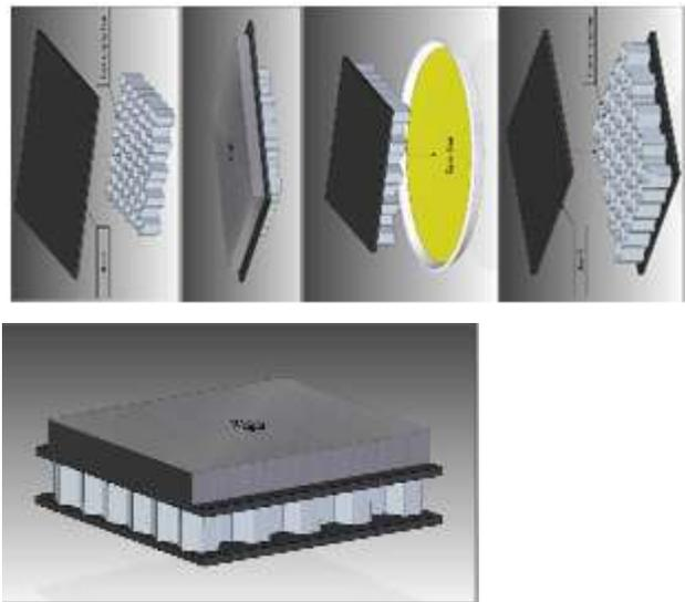
Fig 2.4.2 stages of building of honeycomb structures
