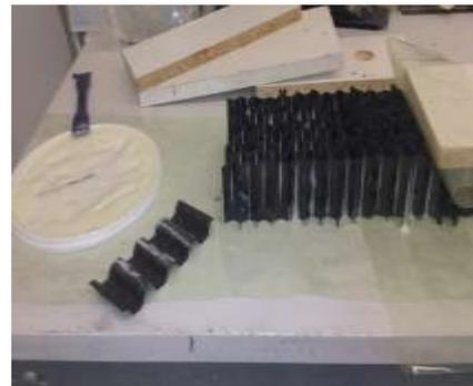
Fig 2.3.2 carbon honeycomb core
