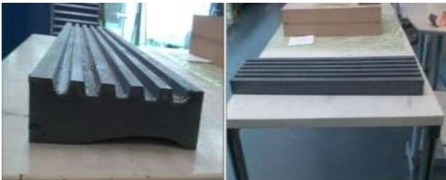
Fig: 2.2.1.1 POM mould for experimental lamination of a layer for honeycomb
