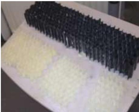
Fig2.2.4 final composite honeycomb core
