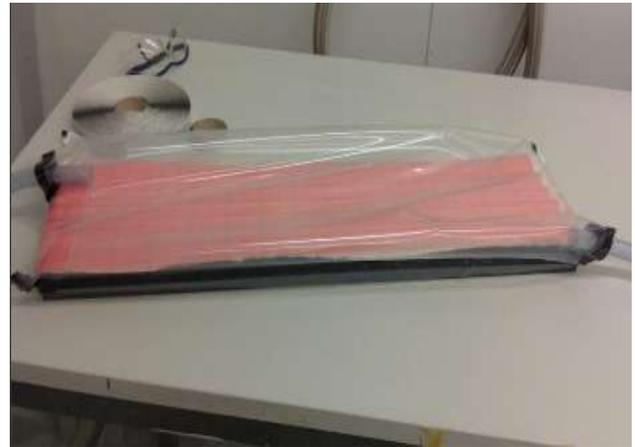
Fig 2.2.1.4 Vacuum impregnation of fiber glass with epoxy resin
