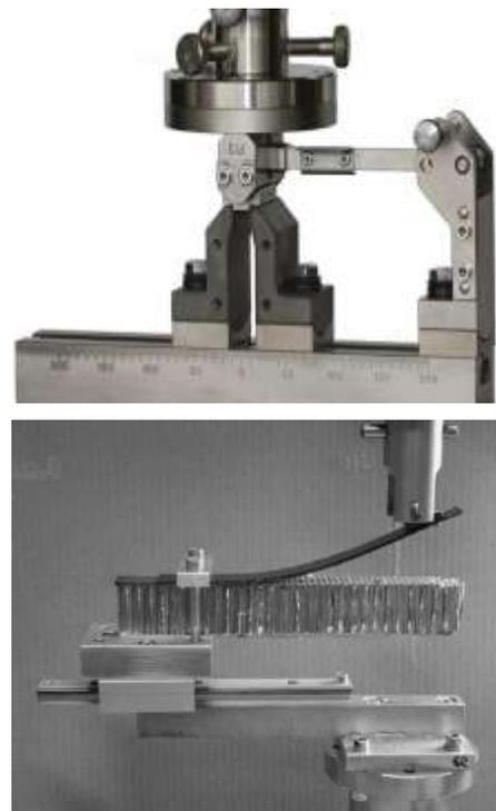
Fig 2.7.1 interlaminar shear strength testing machine
