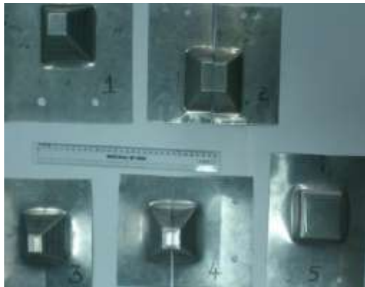
Fig 3.1 Formed Components of AA5052 Sheet Metal
