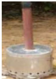
Fig. 1. TLUD gasifier method for biochar production
