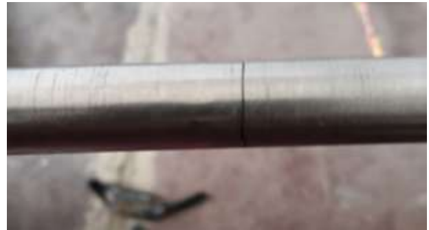
Fig.4 Crack in Rotor Shaft
