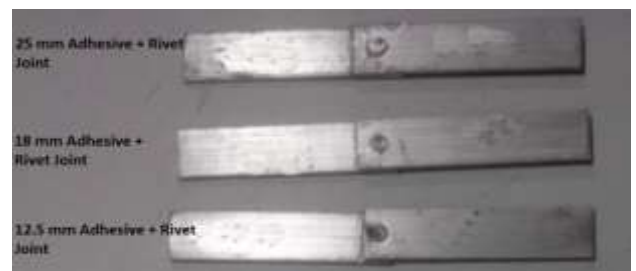
Fig. 10 Actual Specimen of Rivet + Adhesive joint having lap length 12.5mm, 18 mm & 25 mm
