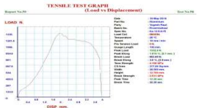
Fig. 11 Load vs. Displacement graph of Adhesive+ Rivet joint having 12.5 mm Lap length.
