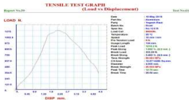
Fig. 7 Load vs. Displacement graph of Rivet joint having 12.5 mm Lap length
