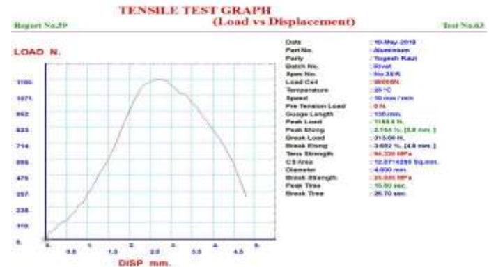
Fig. 9 Load vs. Displacement graph of Rivet joint having 25 mm Lap length.
