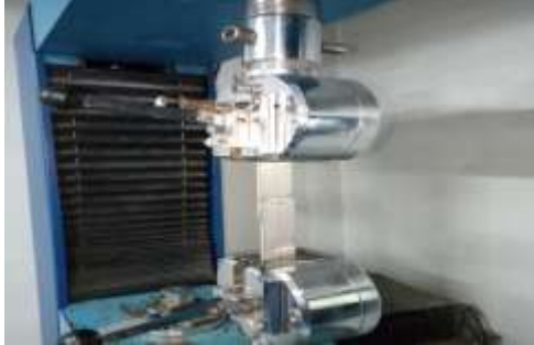
Fig.1 Universal Testing Machine with specimen.
