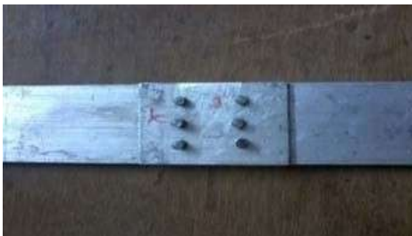
Fig.1. Rivets arranged perpendicular to the loading axis (0°)
