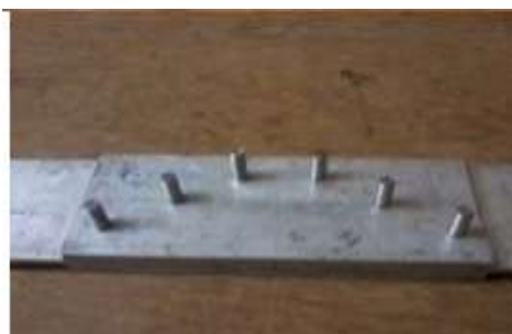
Fig.3. Rivets arranged at 60° from the horizontal axis
