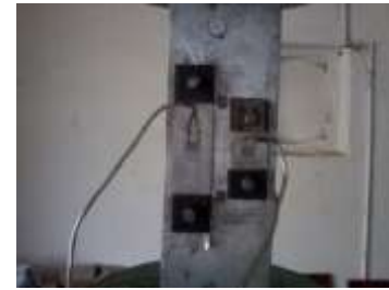
Fig.8. Rivets are arranged in 30° from the horizontal axis
