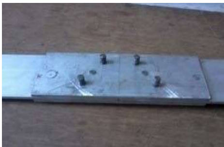
Fig.2. Rivets arranged at 30° from the horizontal axis
