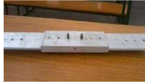
Fig.4. Rivets arranged at 90° from the horizontal axis
