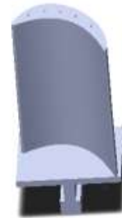
Fig1. Turbine second stage rotor blade with 5 holes
