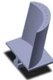
Fig2. Turbine second stage rotor blade with 9 holes
