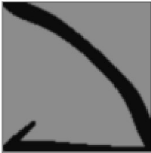
(a) Optimized layout after 500 design iterations, 80% concrete, 20% steel. Black = steel, gray = concrete.
