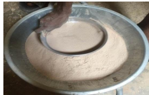
Figure 3: Powdery Ceramic Tiles (After Sieve 75µm)
