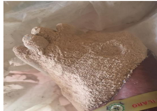
Figure 2: Powdery Ceramic Tiles (Before Sieve)
