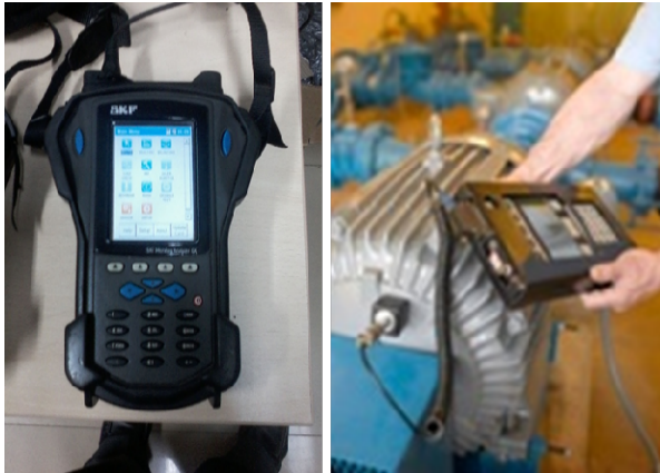
Fig. 7 : Downloading, Measuring & Uploading of data for measurement points into & from SKF Microlog Vibration analyzer
