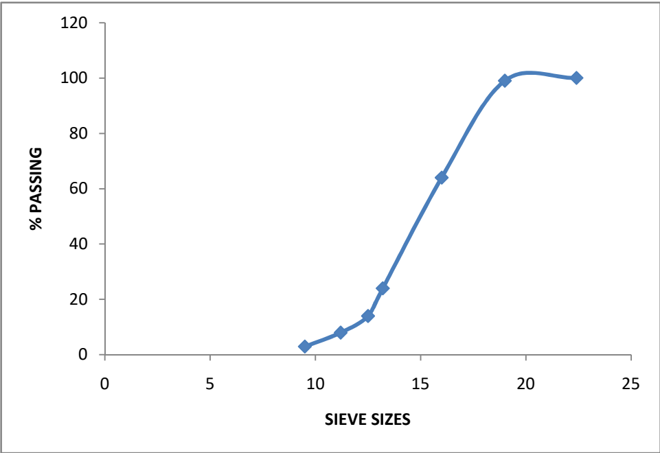
Figure 2 Grading Curve of Coarse aggregate
