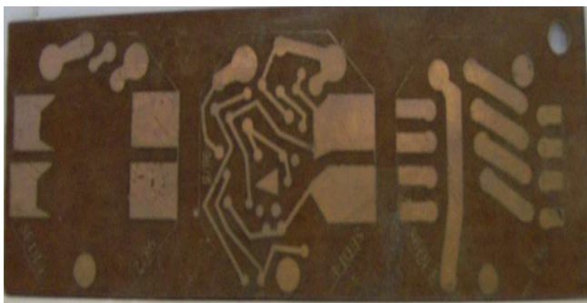
Plate 4: Virgin unpopulated printed circuit board with circuit patterns sketched.
