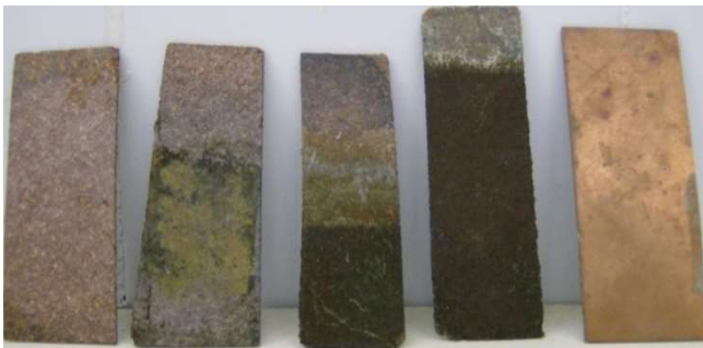
Plate 3: Saw dust boards arranged in increasing order of treatment from unclad to clad
