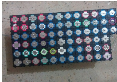
Fig. 9: Series parallel connection of the battery
