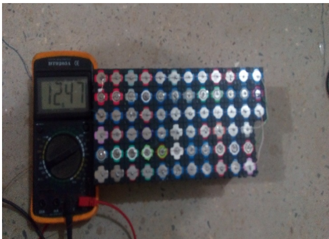
Fig. 11 : Output voltage result of the battery
