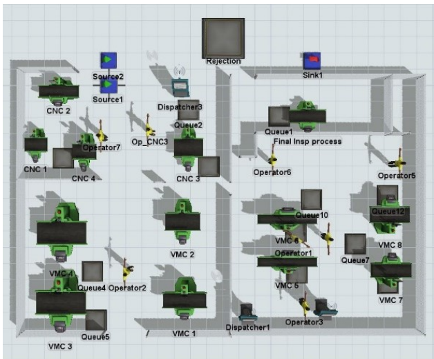
Fig. 3: Conceptual Simulation Model in FlexSim Software.
