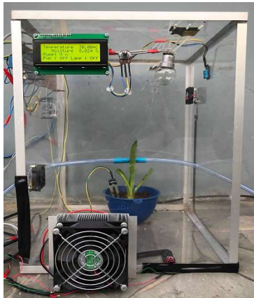
Fig.8. Display for moisture decreasing in soil
