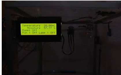
Fig.7. Displaying the sensor value and actuators state inLCD
