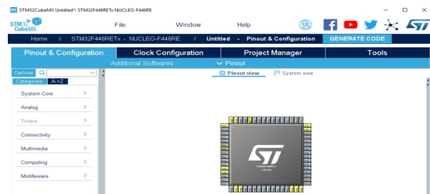
Fig. 6 All pins are cleared from STM32F446RE
