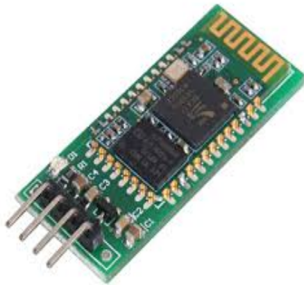
Figure 1. Bluetooth Module HC-05
