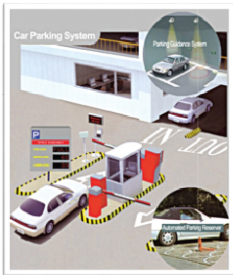
Fig. 1.0: Car park management System using RFID
