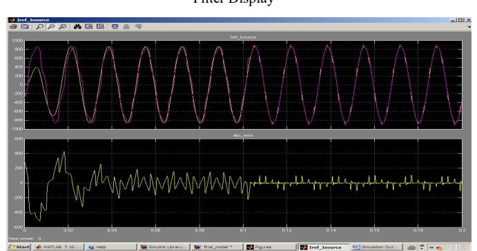
Fig. 18 Average Industrial Load with AHF (a) Reference and Source current and (b) Error
