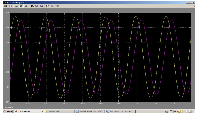
Fig. 8 Voltage and Current Waveforms for AC Load before Compensation
