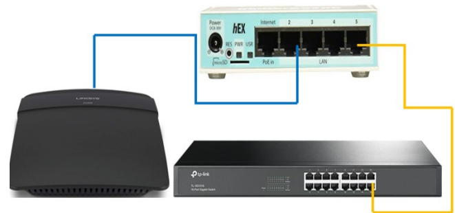
Fig. 3 Cisco Wireless Router, MikroTik Router and TP-Link Switch Connection
