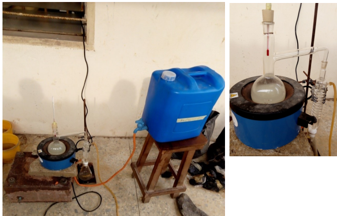
Figure 1: Bio-ethanol distillation Process
