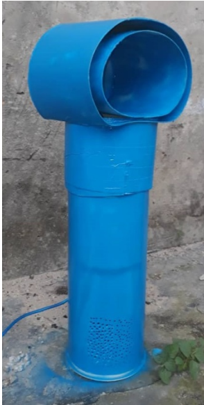
Fig.4.0: the final construction
