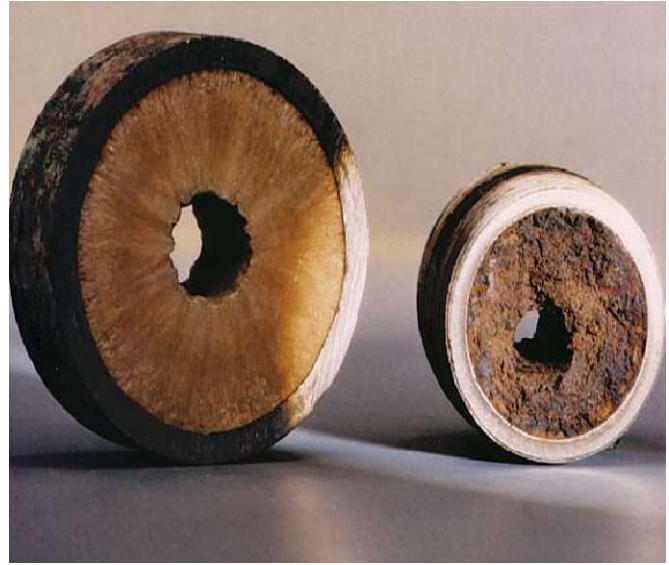
Fig 1. Scale formation in tubing (sandengen, 2006)
