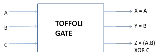
Fig. 2 denotes the basic logic diagram of TOFFOLI Gate
