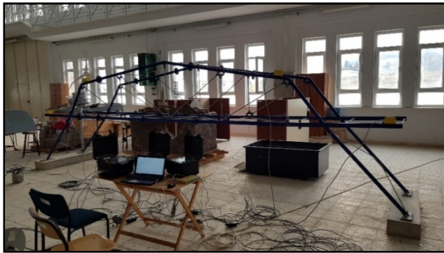
Figure 4. Accelerometer placed on the model steel bridge
