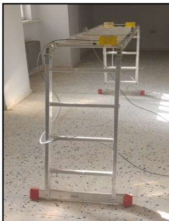
Fig. 2 Bench-Scale Aluminum Bridge
